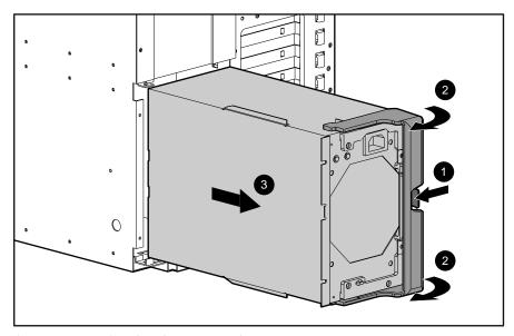
Figure 2-34. Removing a hot-plug power supply
